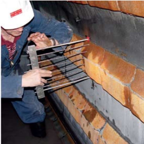
Above: Taking a wear reading for predicting wear life
