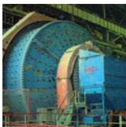
Below: Large SAG mill in the copper industry with some of the local Vulco mill liner team
