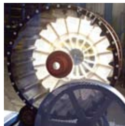
Above: Model mill for optimizing design of grate discharge assembly
