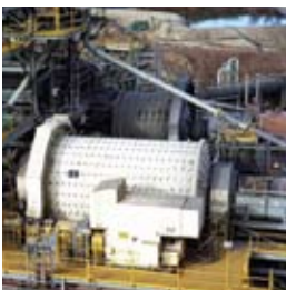
Above top: Metal cap shell plates and lifters plus metal cap lifters on the grate discharge mill end Above bottom: Typical SAG/ ball mill circuit
