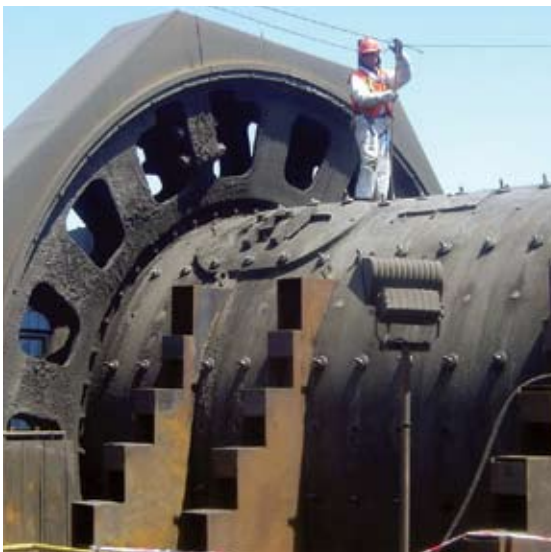
Left: Block type steps and overhead wire for safety during maintenance
